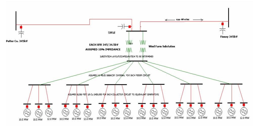
EACH GENERATOR IS EQUIVALENT TO EITHER 7 OR 8 WIND TURBINES (1.5MW EACH) GENERATOR EQUIVALENTS INCLUDE PAD MOUNT XFR CHARACTERISTICS
